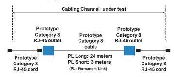
Long Channel: 30 meters, Cords = 3 meters Short Channel: 5 meters, Cords = 1 m
