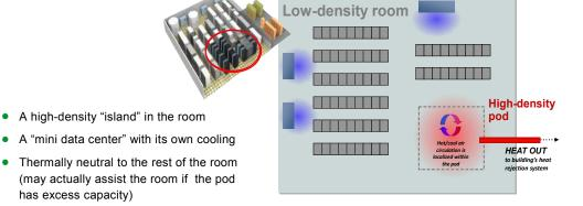
Important basic characteristics of a high density pod include:
